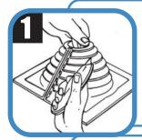
Select an appropriate Master Flash® Standard Retrofit with a pipe range that goes below and beyond fitting. If necessary, follow the lines clearly shown on the flashing and create an opening 10-20% smaller than pipe diameter. For the steep roof slopes or higher corrugation of the profile, bigger size of Master Flash® should be chosen.
