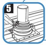
Make a hole in the flange to insert a cable tie or steel band depending on product material.
