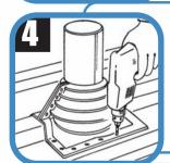
Fix the flashing using self-drilling screws. Spacing between fasteners must not exceed 38mm (1.5").
