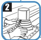
Wrap Master Flash® Retrofit around the pipe. Press the flashing down, bending it to conform to roof profile or irregularities. A blunt tool will help to form flashing to tight roof angles.
