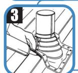
Apply sealant between the base roof and at the top of the flange.
