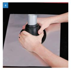
Slide the Master Flash® Residential down the pipe, using a non-petroleum-based lubricant to ease installation.
