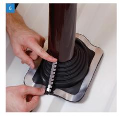
Place the stainless steel gripper on the flange to close and secure the Master Flash  $^{\! \circ}$  Multi-Flash.
