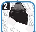
Slide the Master Flash® Extreme Angle down the pipe, using a non-petroleum-based lubricant to ease installation.
