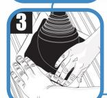
Press Master Flash® Extreme Angle down, bending it to conform to roof profile or irregularities. A blunt tool will help to form flashing to tight roof angles.
