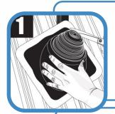
Select an appropriate Master Flash® Extreme Angle with a pipe range that goes below and beyond fitting. If necessary, use the lines clearly shown on the flashing to trim an opening 10-20% (5-10% for Retrofit applications) smaller than the pipe diameter.
