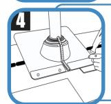
Fix the flashing to the roof using nails, then cover the upper part of the flashing with roofing tiles.
