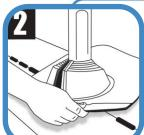
Wrap the Master Flash® around the roof penetration. Press Master Flash® down, bending it to conform to roof profile or irregularities. A blunt tool will help to form flashing to tight roof angles.
