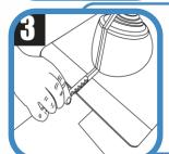
Install stainless steel gripper to close the previously cut seam.
