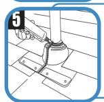
Additional sealant may be applied between the flashing and the pipe. Apply as needed.
