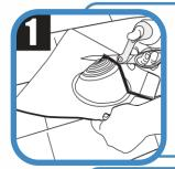
Cut the flashing down the seam. If necessary, use the lines clearly shown on the flashing to trim an opening 5 - 10% smaller than pipe diameter.
