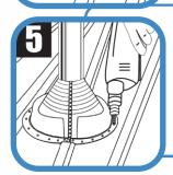
Fix the flashing using self-drilling screws. Spacing between fasteners must not exceed 38mm (1.5").
