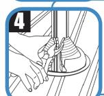
Install the stainless steel gripper to seal the flange.
