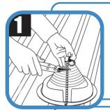
Select an appropriate Master Flash® Universal Retrofit with a pipe range that goes below and beyond fitting. If necessary, follow the lines clearly shown on the flashing and create an opening 5-10% smaller than pipe diameter. Slice down the flange. For the steep roof slopes or higher corrugation of the profile, bigger size of Master Flash® should be chosen. If using this product as a Retrofit, cut down the side in the clearly-marked flange.
