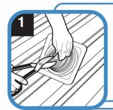
Select an appropriate Master Flash® Standard with a pipe range that goes below and beyond fitting. If necessary, use the lines clearly shown on the flashing to trim an opening 10 - 20% smaller than pipe diameter. For the steep roof slopes or higher corrugation of the profile, bigger size of Master Flash® should be chosen.
