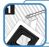
Select an appropriate Master Flash® Retrofit with a pipe range that goes below and beyond fitting. If necessary, follow the lines clearly shown on the flashing and create an opening 10-20% smaller than pipe diameter. Slice down the flange. For the steep roof slopes or higher corrugation of the profile, bigger size of Master Flash® should be chosen.
