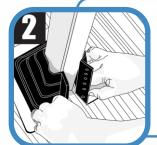
Wrap Master Flash® Square Vent around the pipe and install all snap rivets to seal the flange.
