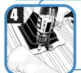
Use fasteners to complete sealing. For installation, fastener spacing must not exceed 38 mm (1.5").
