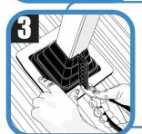
Press Master Flash® down, bending it to conform to roof profile or irregularities. A blunt tool will help to form flashing to tight roof angles.
