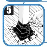
Make a hole in the flange to insert a cable tie or steel band depending on product material. Slide the cable tie through the hole, ensuring that it is resting on the flashing. Put the cable through the hole to assure tight fitting. Additional sealant may be applied between the flashing and the pipe. Apply as needed.
