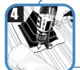
Use fasteners to complete sealing. For installation, fastener spacing must not exceed 38 mm (1.5").
