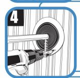
Use fasteners to complete sealing. For a secure installation, fastener spacing must not exceed 38mm (1.5").
