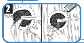
Wrap the Master Flash® Multi Low Profile around the pipe, bending it to conform to roof profile or irregularities. A blunt tool will help to form flashing to tight roof angles. Apply sealant between the base of the flashing and the roof.
