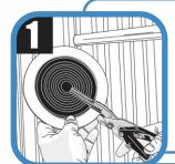
Select an appropriate Master Flash® Low Profile Multi Flash with a pipe range that goes below and beyond fitting. If necessary, use the lines clearly shown on the flashing to trim an opening 5-10% smaller than the pipe diameter. For retrofit applications cut the flashing along the marked seam.
