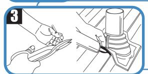
Trim the stainless steel gripper to match the size of the cut flashing. Apply sealant between the base of the flashing and roof and at the top of the flange.
