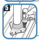
Fix the flashing to the surface using self-drilling screws assembled with washers. The spacing between the screws should not exceed 38 mm (1,5 inch.).
