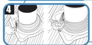
Crimp the previously cut flange with the gripper. Apply additional sealant on the seam if necessary.
