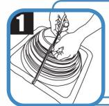
Select an appropriate Master Flash® Retrofit with a pipe range that goes below and beyond fitting. If necessary, follow the lines clearly shown on the flashing and create an opening 5-10% smaller than pipe diameter. For the steep roof slopes or higher corrugation of the profile, bigger size of Master Flash® should be chosen. If using this product as a Retrofit, cut down the side in the clearly-marked seam.
