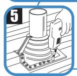
Use fasteners to complete sealing. For installation, fastener spacing must not exceed 38 mm (1.5").
