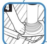
Apply sealant between the base of the flashing and the roof.
