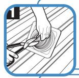
Select an appropriate Master Flash® Multi Standard with a pipe range that goes below and beyond fitting. If necessary, use the lines clearly shown on the flashing to trim an opening 10 - 20% smaller than pipe diameter. For the steep roof slopes or higher corrugation of the profile, bigger size of Master Flash® should be chosen.
