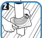
Slide the Master Flash® down the pipe, using a non-petroleumbased lubricant to ease installation.
