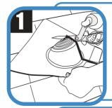
Select an appropriate Master Flash® Electrical Mast Connection. Cut the flashing down the seam. If necessary, use the lines clearly shown on the flashing to trim an opening 20 - 30% smaller than pipe diameter.
